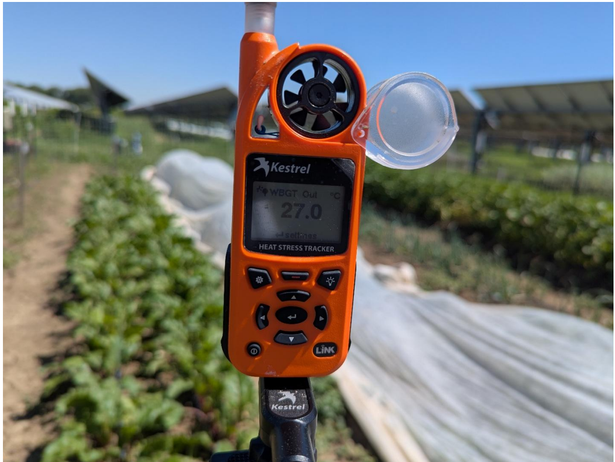
Figure 3: A sensor showing the Wet Bulb Globe Temperature in the full sun (traditional open field agriculture) at 11am at Jack's Solar Garden, Longmont, CO
