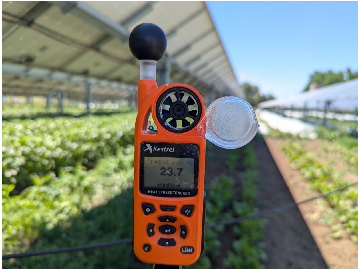
Figure 2: A sensor showing the Wet Bulb Globe Temperature in the shade created by the solar panels at 11am at Jack's Solar Garden, Longmont, CO
